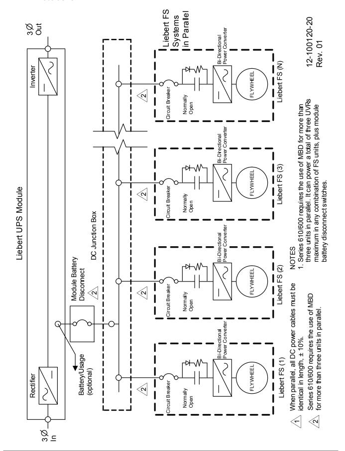
Figure 142One-line diagram, single Liebert FS and battery with factory-integrated circuit breaker supplying Liebert UPS—UPS DC terminal point of common connection
